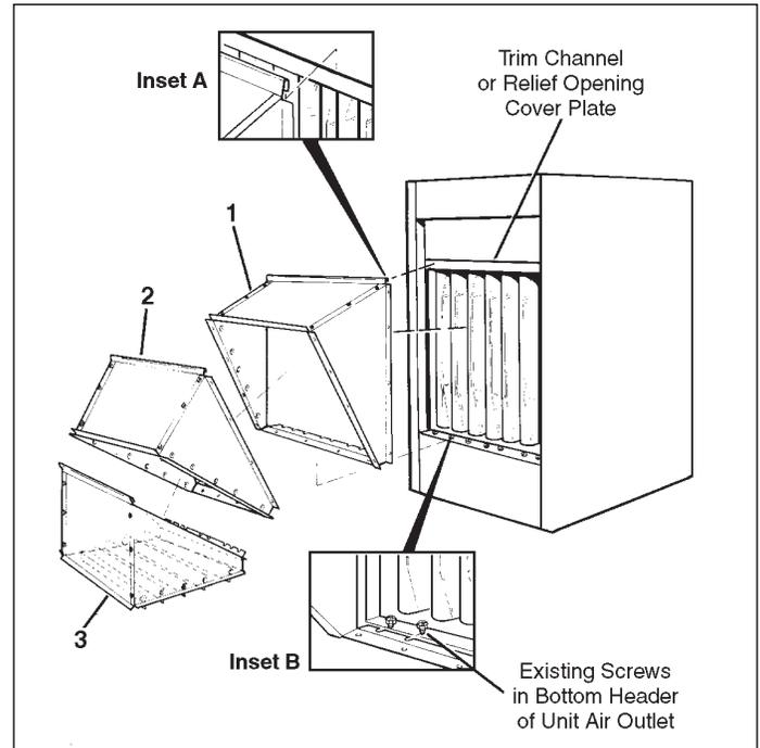
To remove the spring loaded louver blades, simply apply pressure against the louver blade retaining spring by grasping the blade and forcing the blade to the left as you face the unit heater. After compressing the spring, the right hand tab of the louver blade can be removed from the unit, and then the spring end of the blade removed.
