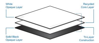
Virgin Grade Outer Layer Resins = Stable Outdoor Exposure Recycled Core Resins = Economical Green Alternative Tri-layer Construction = Excellent Tear & Puncture Strengths
